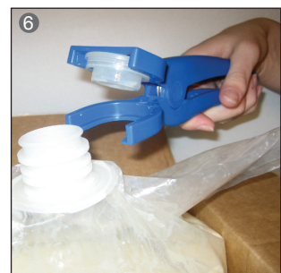
Remove Quick Up and leave the cap in the Quick Up, if the cap should be used for reclosing the bib.
