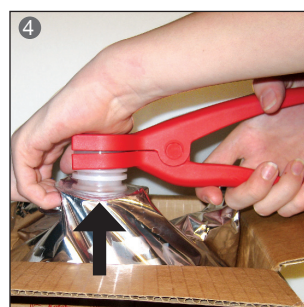
IMPORTANT: lift the bag to secure no liquid in the top of the bib to avoid spurting.
